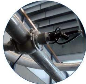
Fig. 1: M1100 sensor in use between tank and filler in a 60 mm line.
